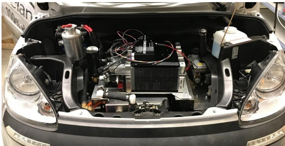
Figure 6 – Hydrogenics fuel cell system integrated into elano former motor compartment.
