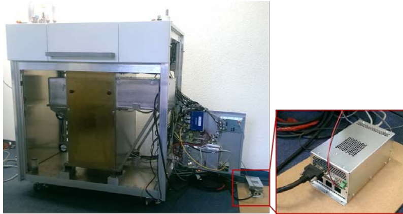
Figure 19: Prototype of the high-energy microCT system. The magnification shows the controller board that had to be developed for controlling the detector and for retrieving the acquired images. Some specification of the controller are given in the table.
