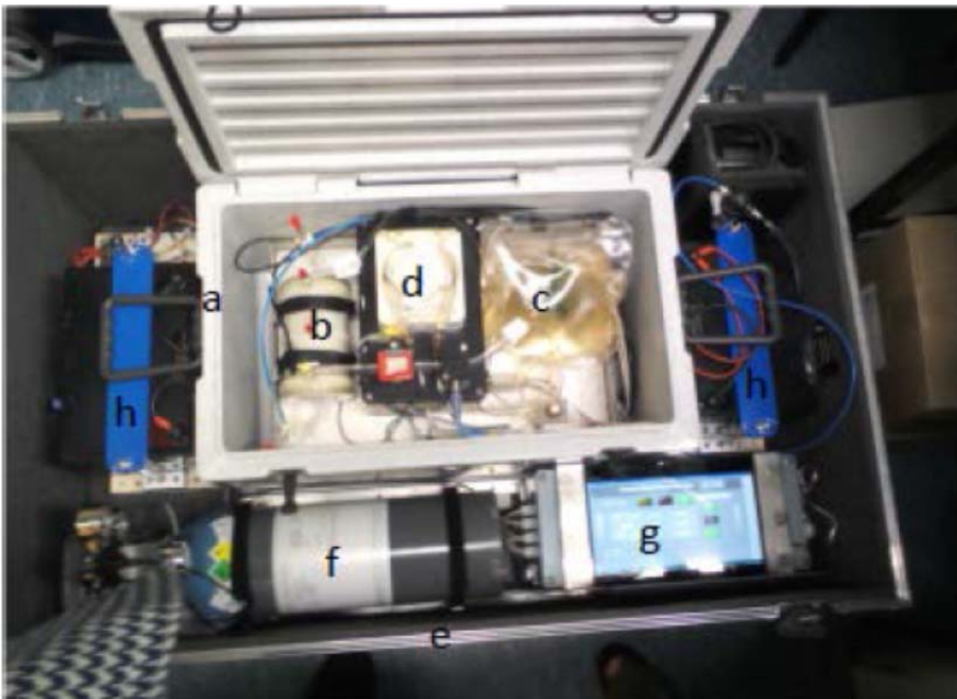
Figure 3: Top view of the transport box with visibly the (a) inside box containing (b) bioreactor, (c) medium bag, (d) medium pump, and (e) the outside box containing (f) gas cylinder, (g) computer, and (h) batteries.
