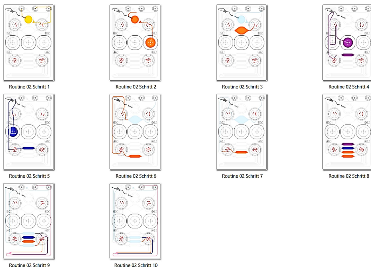
Figure 4: Sequence of operating routine cartridge where turning valves integrated on the chip are controlled via the reader to activate fluid streams as required. On chip blisters with stored reagents are punched in a precise sequence to ensure delivery of reagents as needed in the carefully timed on-chip reactions (MFCS, example from early-generation chip concept.)
