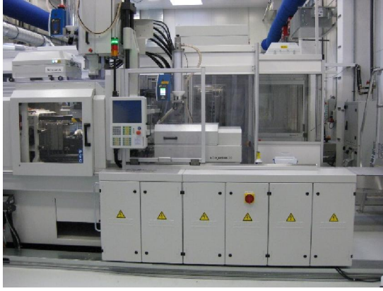
Figure 2: (left) Injection molding machine at microfluidic ChipShop, (right) Fully processed, closed ROUTINE 02 chip with blisters, turning valves and syringes. The chip measures 75x50mm, i.e. double glass slide format, which is an industry standard.
