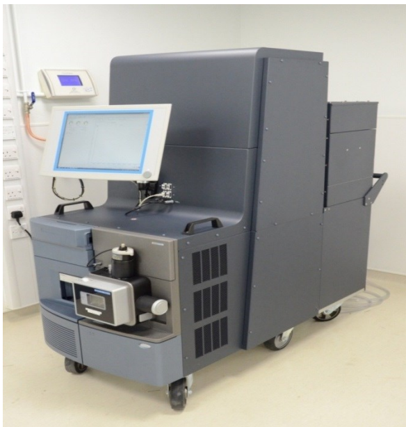
4. Figure Mass Spectrometric pre-prototype device, surgical version. (Xevo G2S)
