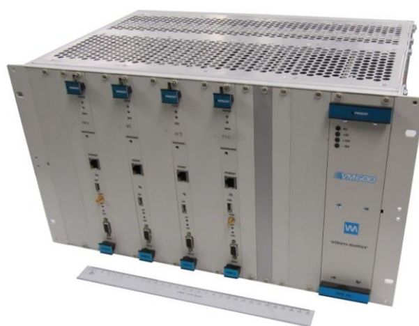
Figure 17: VM600 rack with processing cards
