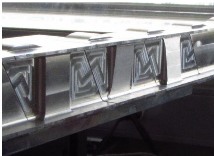
Figure 3: The three ribs prototypes for joint measurement of clearance and axial position
