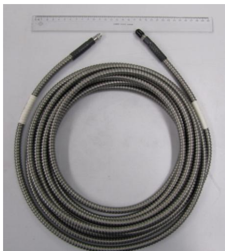
Figure 16: Extension cable (7m)
