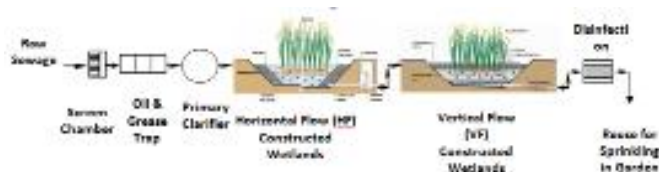
Fig. 68: Treatment schematic diagram at Dayanand Park site
