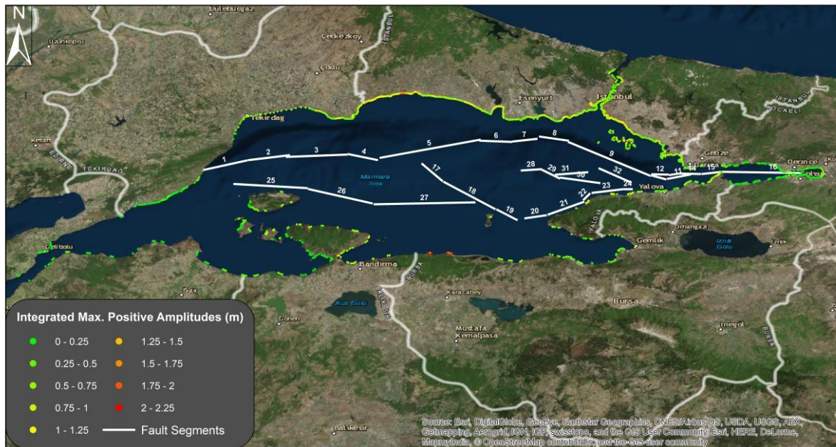
Figure 15: The distribution of calculated maximum wave amplitudes at each gauge points for all earthquake scenarios.
