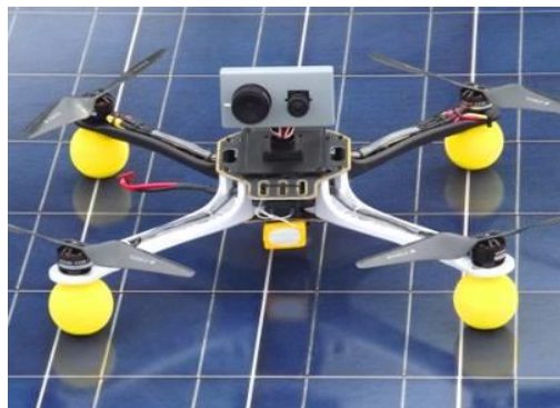
Figure 22. Testing kits: First version of the developed quadcopter (PV drone). It has an IR camera and a visible camera for monitoring a PV installation.
