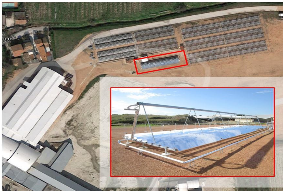
Fig. 1.19 The collector field installation in Soltigua's industrial site Laterizi Gambettola in Italy. The framed area indicates the monitored collector field, which is also shown in the inset picture.
