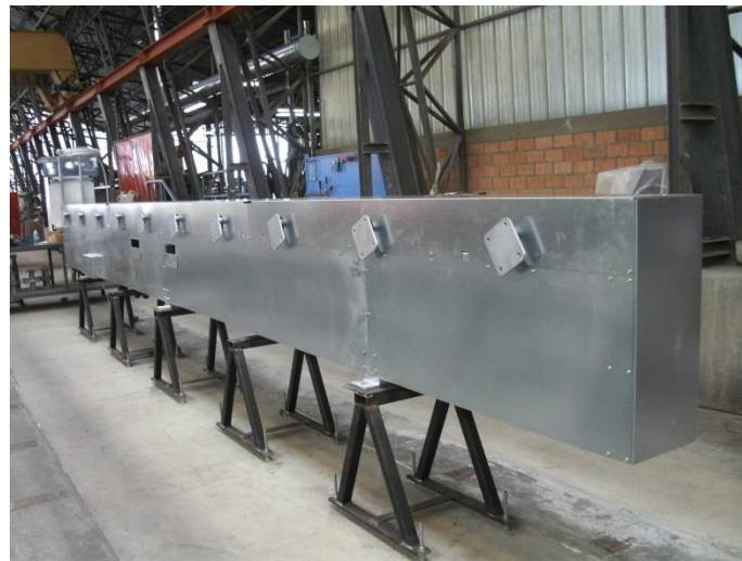
Fig.1.5 FRESH NRG prototype drive ready to be shipped to Fraunhofer ISE for the lab prototype test. The connections of the mirror beams are visible in the front.
