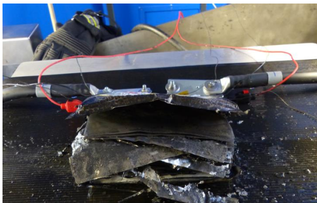
Figure 11: The effect of performing an overcharge on one of the selected cells
