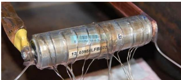
Figure 16: Cell, equipped with 13 temperature sensors
