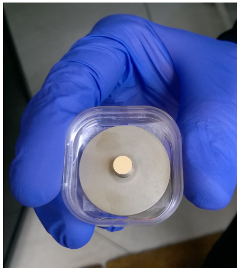
Fig. 22. Single-crystal molybdenum anode substrate that successively hosted dielectric microspacers.
