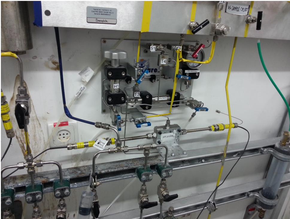
Figure 7: Transfer line for the measurement of the partial pressure of the CO 2 and the pH of the water in the high pressure sample.
