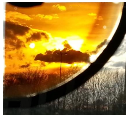
Figure 15: 1.5- \mu\text{m} -thick epi-PECVD silicon foil transferred to glass by anodic bonding.
