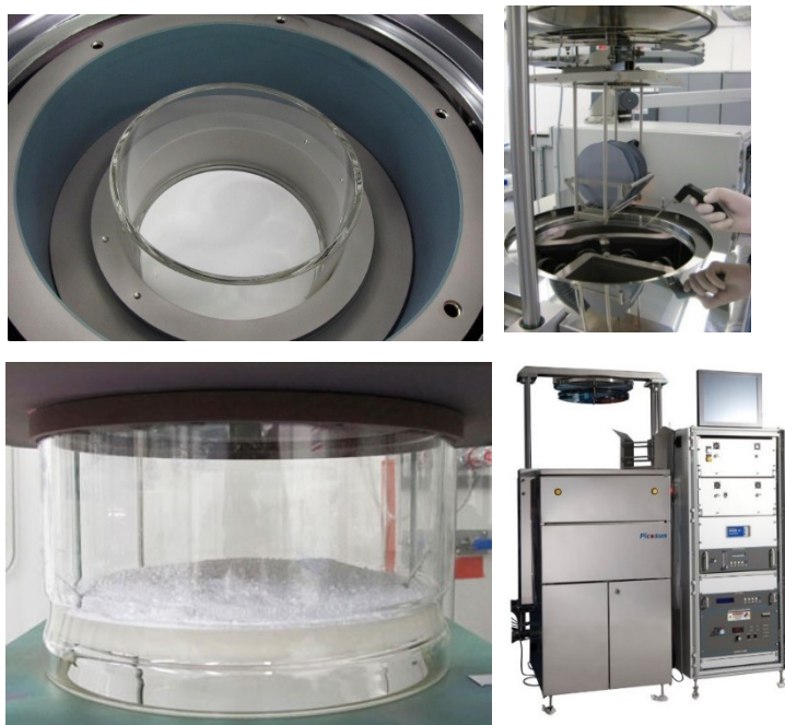
Figure 8: ALD reactor constructions (POCA™ 200 & POCA™ 300) for modification of larger amounts of powders (<500 g)
