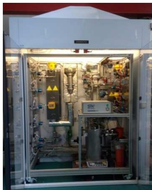
Figure C-10: Overview of the fluidized-bed reactor and of the test bench
