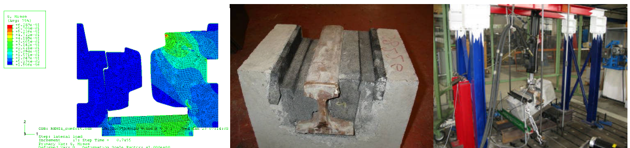
FEM representation of REMS behaviour under load and example of test block and setup
