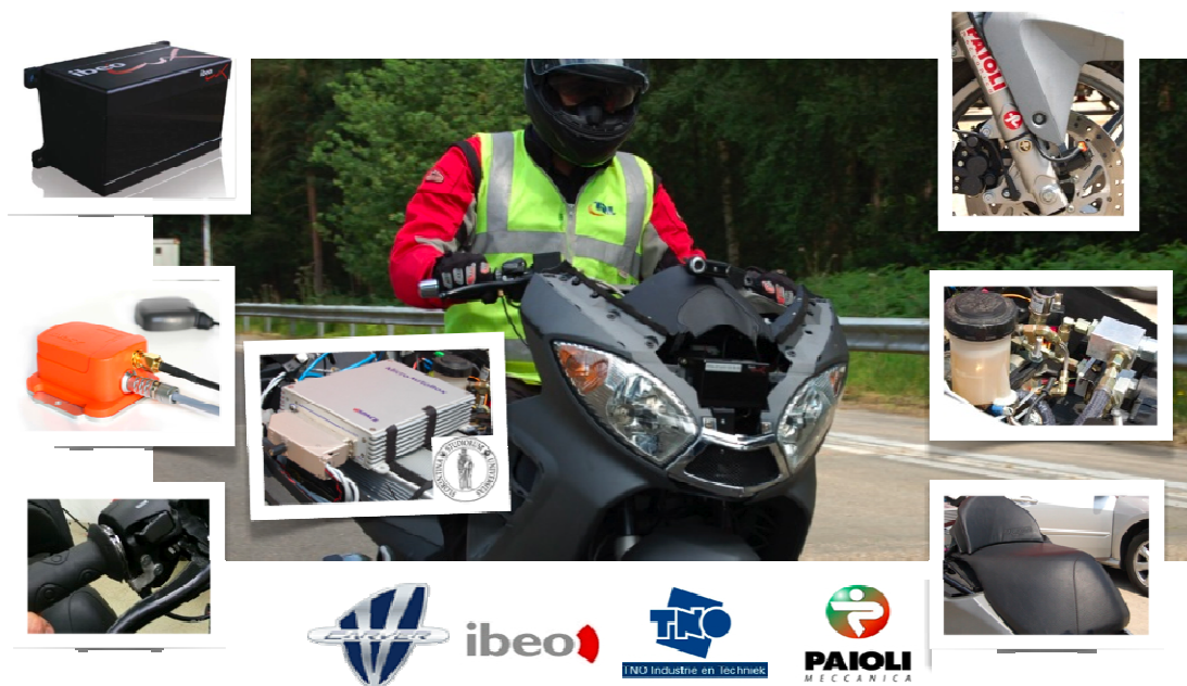
Figure 12: Malaguti test scooter with integrated sensors, actuators and control unit
