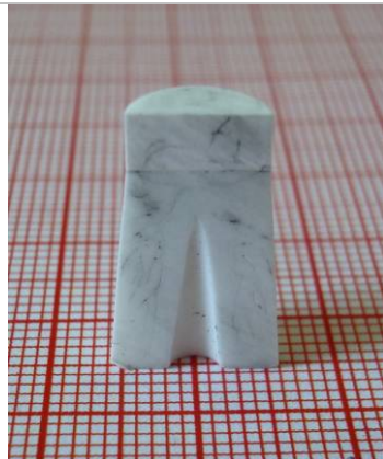
Fig. 3 Cross cut through a braking pad in the sintered state
