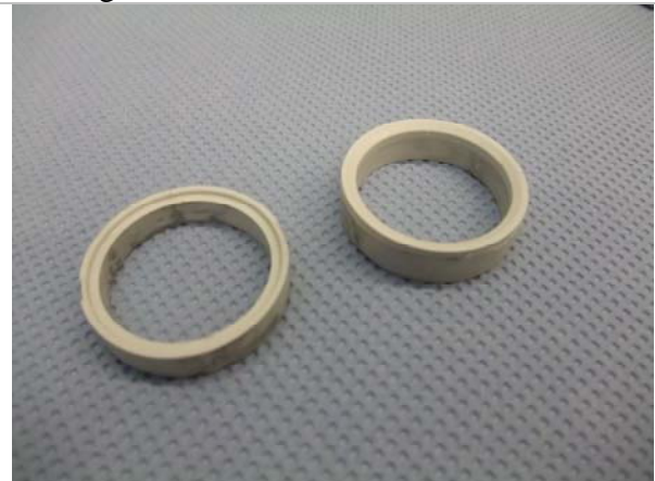
Fig. 4 First component and completed valve seat in the green state
