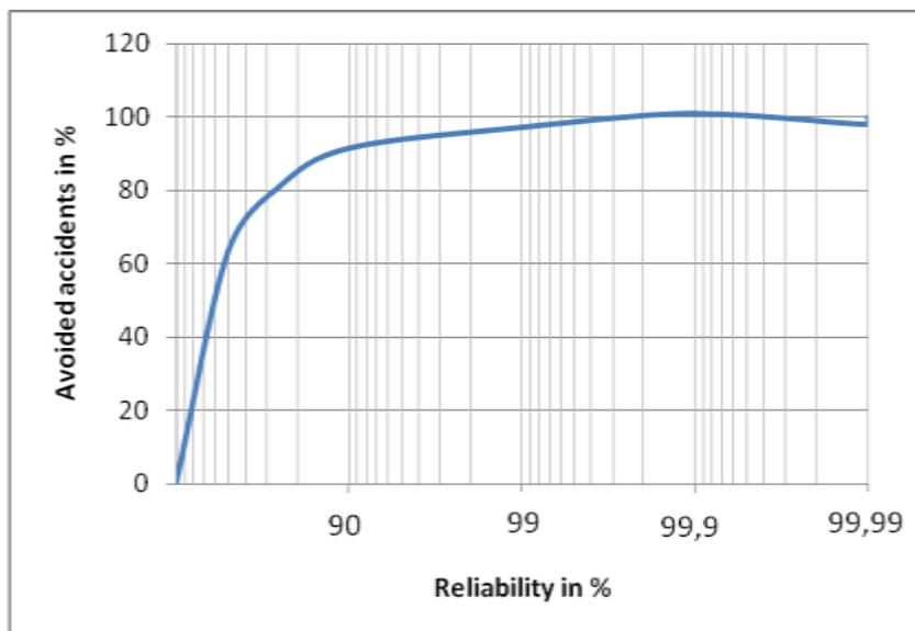
Figure 13 Relative proportion of avoided accidents to reliability of obstacle detection
