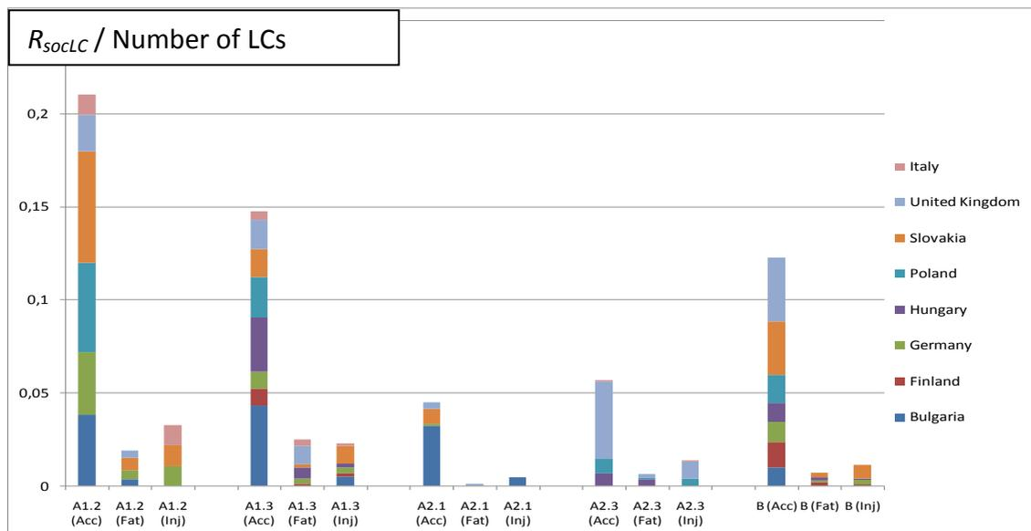
Fig. 6. Comparison of accident statistics at different types of level crossings scaled by level crossing type population (EU).
