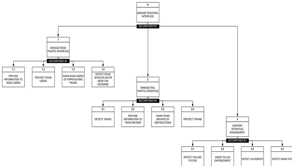
Figure 7 Upper layers of generic functional model of level crossing
