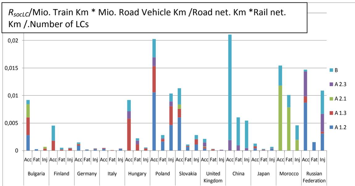
Fig. 5. Comparison of accident statistics scaled by vehicle interactions
