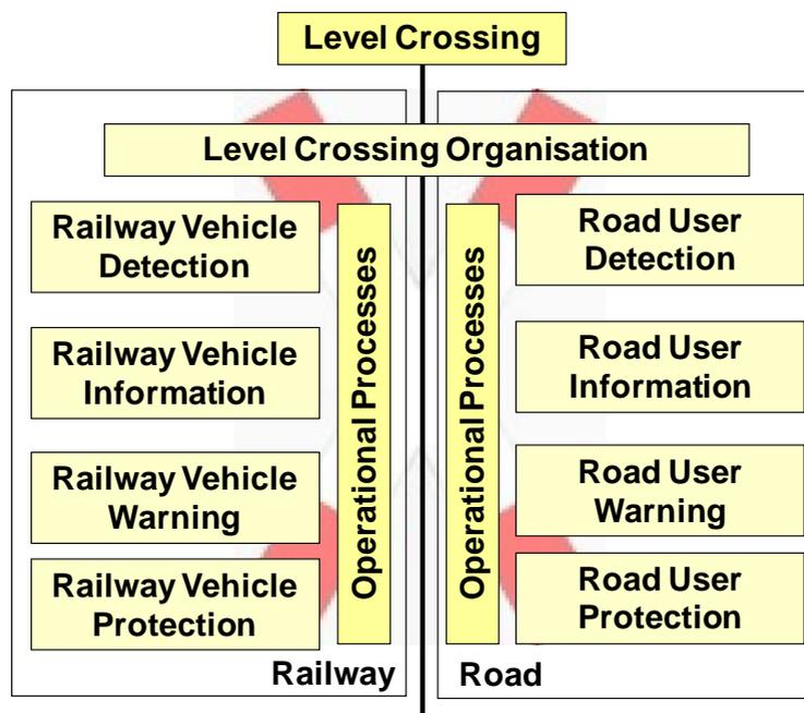
Fig. 3. Functional decomposition of a level crossing system
