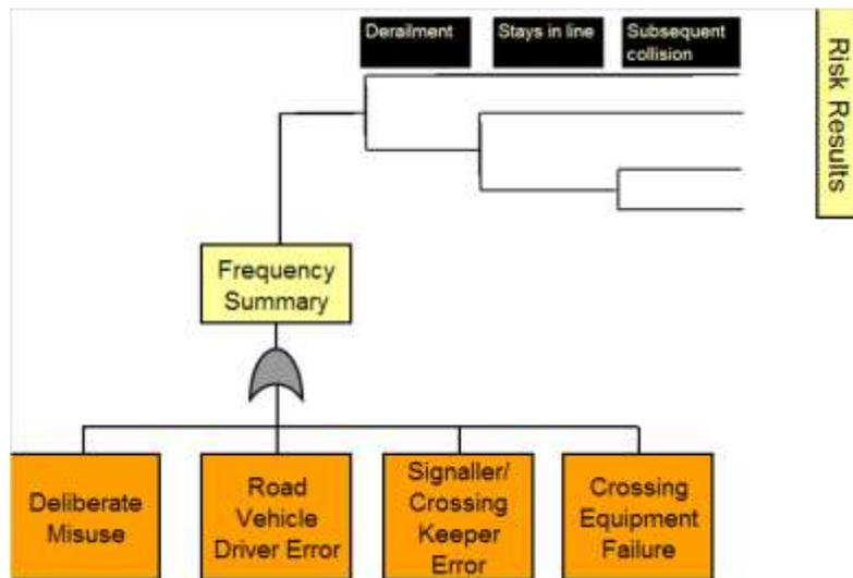
Figure 12 Illustration of the three main elements of the SELCAT level crossing risk model
