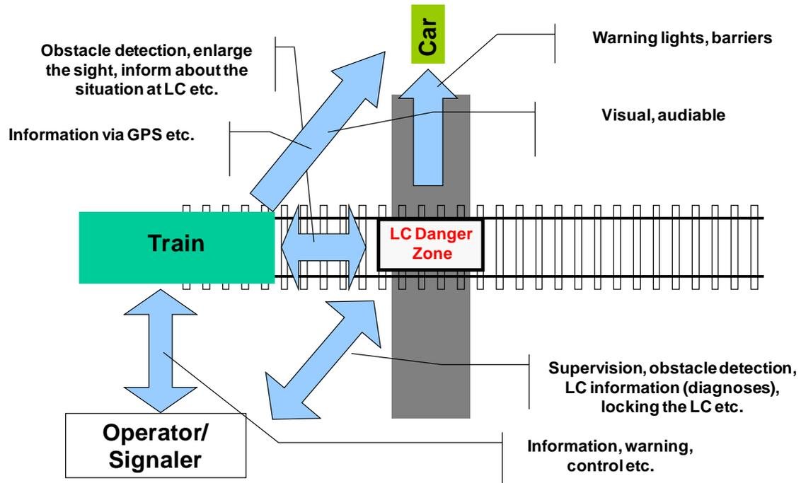
Figure 10. The basic actors and interfaces on a level crossing
