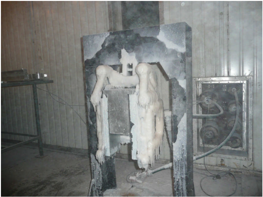
Figure 9 - Testing a Disc Brake Unit at -40°C
