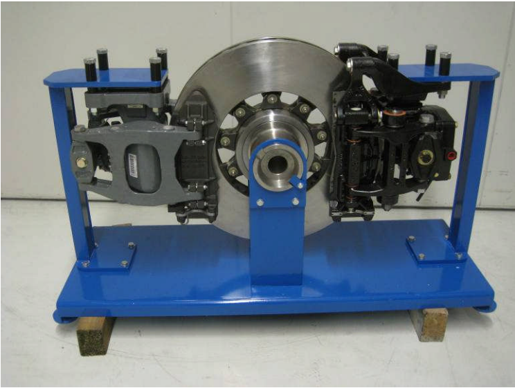
Figure 8 - Mock-up for the mechanical interoperability
