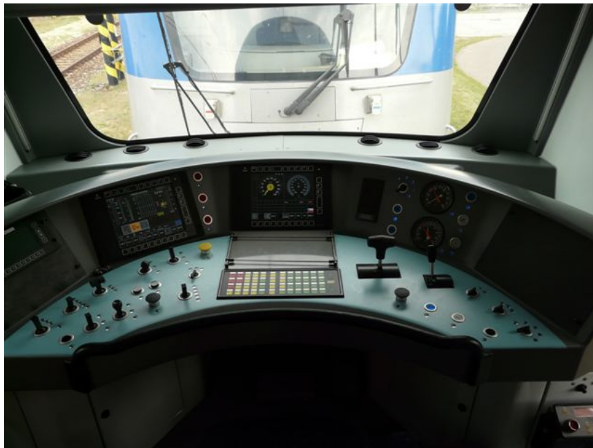
Fig. 3: Design of the driver's desk of the Škoda 109E locomotive prototype based on EUDD principles
