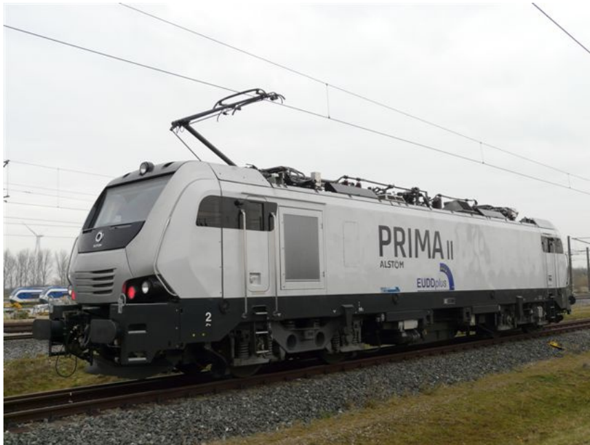
Fig. 7: PRIMA II locomotive prototype used for the in-field tests at Wildenrath test centre
