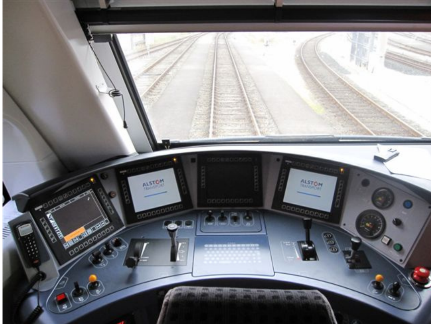
Fig. 8: Left side oriented EUDD plus desk integrated into the PRIMA II locomotive prototype
