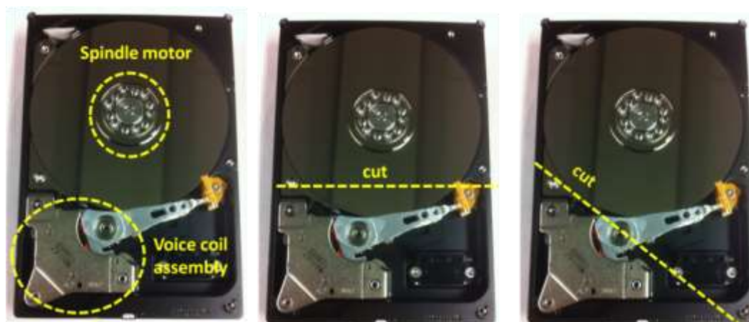
Figure Left: Sintered NdFeB magnet(s) are found in the voice coil assembly and a bonded NdFeB magnet is located in the spindle motor. Middle: A transverse cut (aligned with the short side of the HDD) would put less requirement on the alignment of the HDDs. Right: A biased cutting angle minimizes the amount of aluminium casing that remains attached to the voice coil assembly
