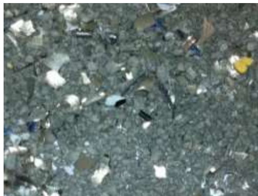
Figure Collected material that passes through the holes in the porous drum after the HD reaction
