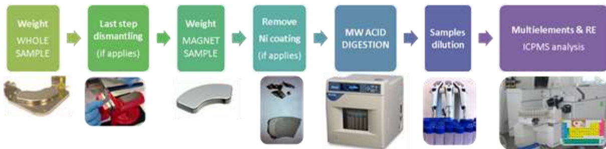
Figure: Schematic description of the ICPMS analysis experimental method for the complete characterization of the magnet samples.
