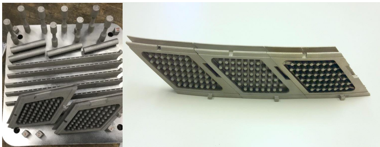
Figure 4.6f Demonstrators and test specimens manufactured from Selective Laser Melting
