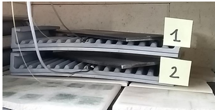
Figure 4.6n: Left Phase response of a F-P sensor embedded in a GE heat shield component under thermal cycling from ambient to 800 °C. The phase scales as a 2nd order polynomial with temperature. (Phase = -3.16 + 9.0 \cdot 10^{-3} \cdot T + 3.60 \cdot 10^{-6} \cdot T^2 ; confidence value R^2=0.9998 ); Right: Heat shields installed in furnace for temperature testing to 800°C
