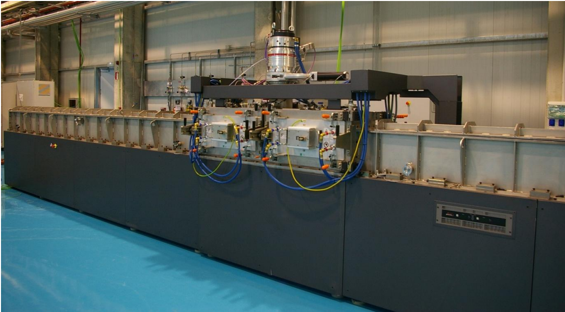
Figure 1. Sputtering chamber used to deposit the solar selective coatings.
