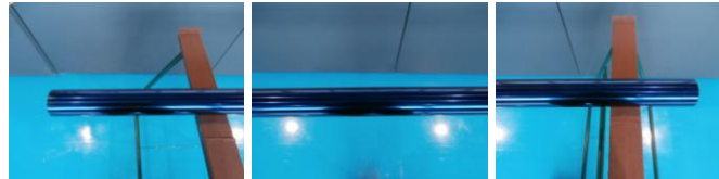
Figure 3. Images of the left, center and right positions of the tube coated with the absorber showing a homogeneous distribution of the color.
