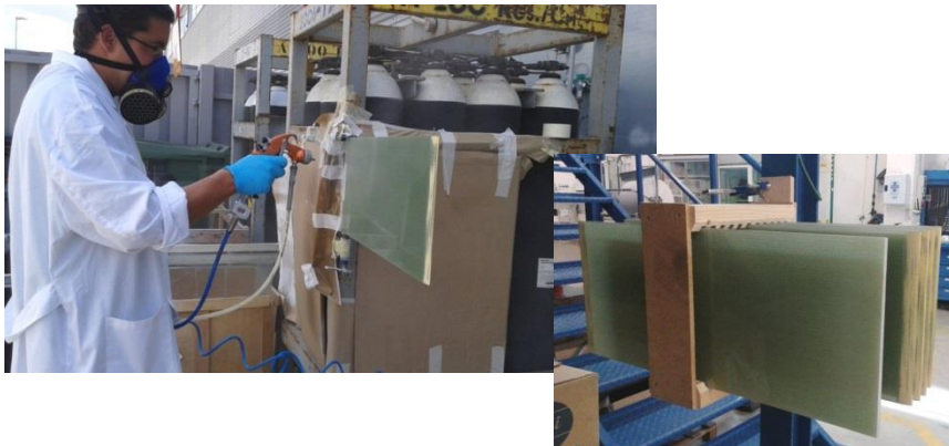
Figure 4 Optimised spray process for flat lab test substrates (Top) and wind turbine blade sections (Bottom)
