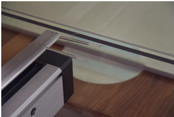
Figure 14 Boundary layer and freestream hotwire probes (a) during insertion into probe support outside the test section, (b) during measurements in the boundary layer
