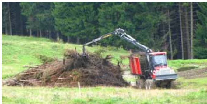
The new high-speed forwarder loading residues in its biomass cradle.
