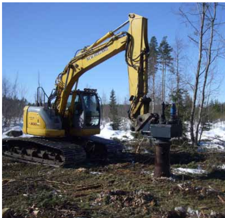
The Ellettari stump extractor is designed for fitting to farm tractor, but here mounted on an excavator.
