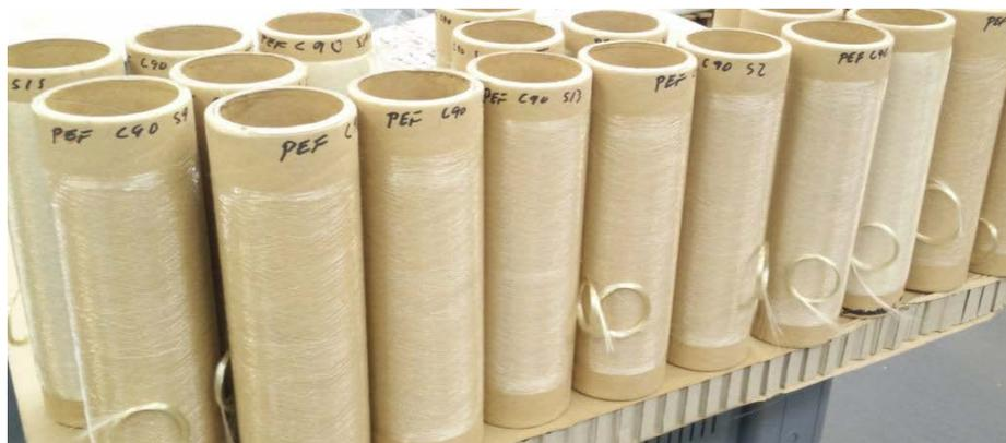
**Figure 2:** Fibres prepared by Lankhorst Euronete from PEF provide by Avantium
