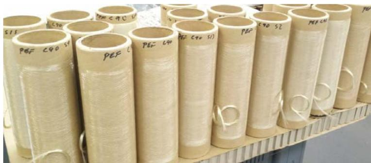
**Figure 3:** Fibres prepared by Lankhorst Euronete from PEF provide by Avantium
