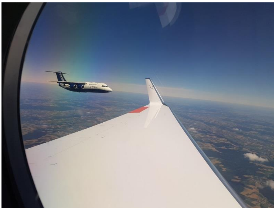
JRA2-TGOE: UK BAe146 aircraft observed from DLR HALO during formation flying to provide an in-flight instrument comparison during EMERGE-EU (2017, Munich)
