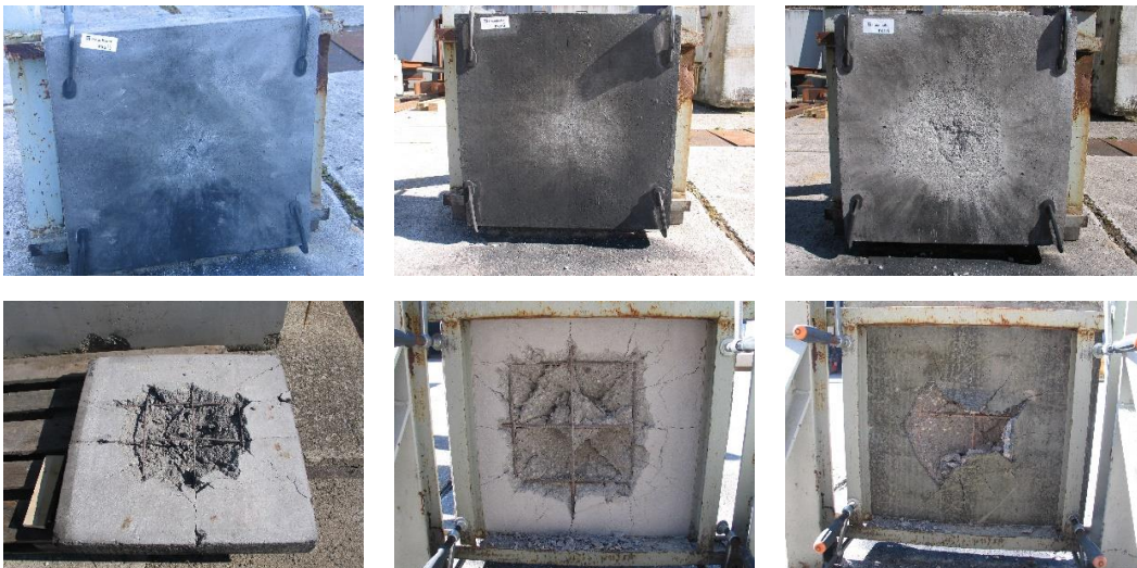
Figure 18 Damaged Elements after detonation tests, above: front face, below: rear face.
