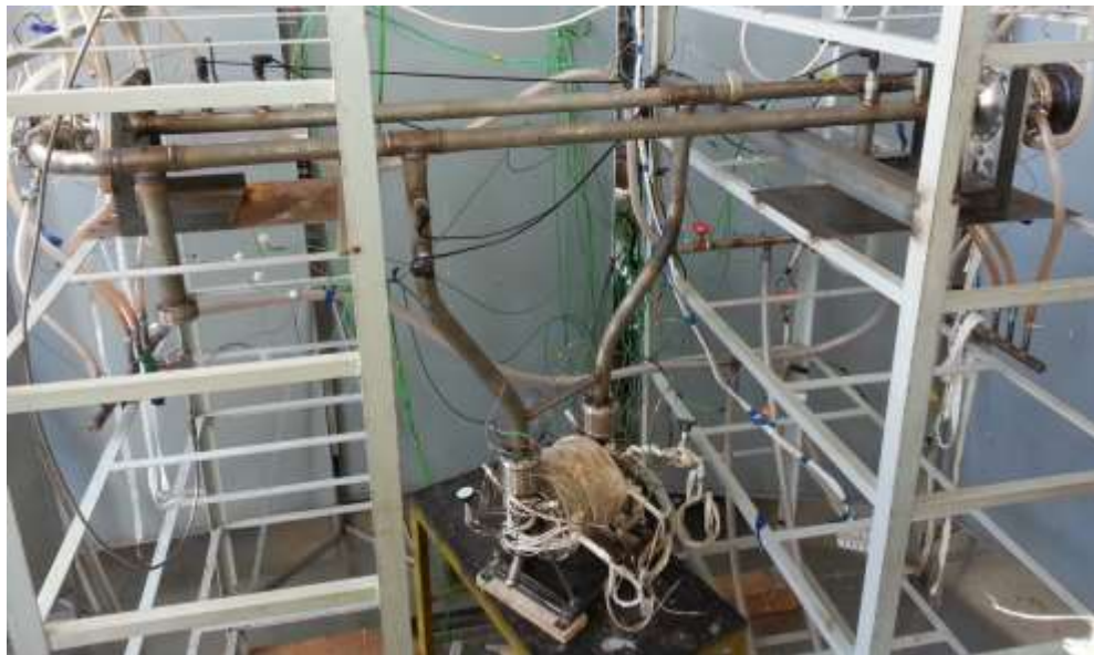
Figure 70: The facility after assembly of TAC loop and MHD generator
