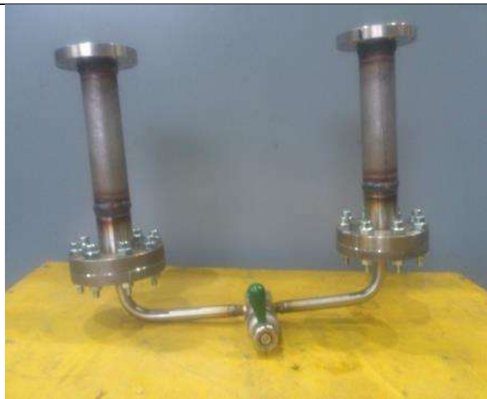
Figure 47: second system of connection between the two part of the thermo acoustic loop. The valve allows adjusting the hydraulic losses.
