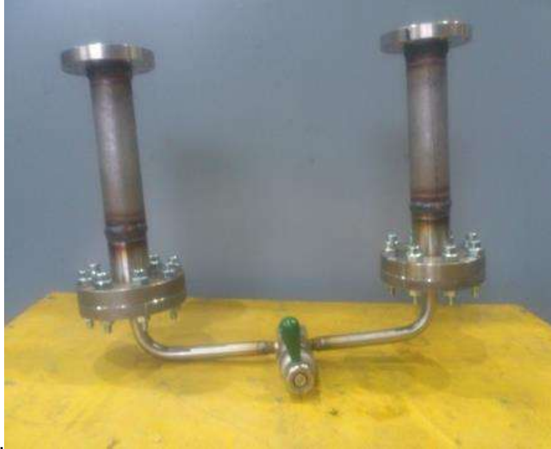
Figure 17: Experiment with hydraulic resistance on the ends of the TAC generator
