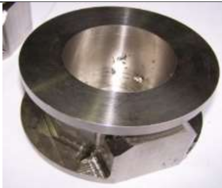
Figure 34: Inconel shield It's made also from Inconel steel and it serves as shield for hot heat exchanger
