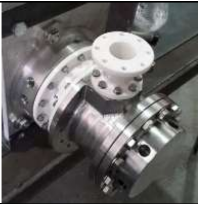
Figure 32: Zirconium connection and Zirconium flange This part, together with Zirconium flange, is made from a special Zirconium Oxide ceramics. Ordered and manufactured in China. Zirconium connection separates a hot part of TAC generator from feedback tubes, so heat cannot go away from TAC generator
