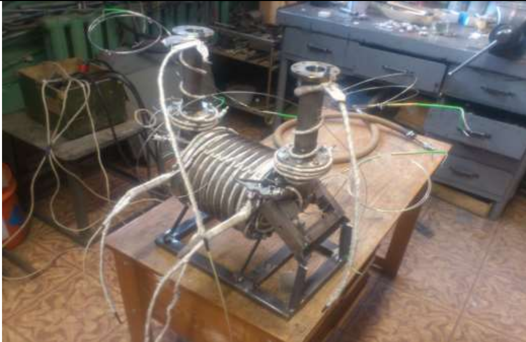
Figure 40: The MHD generator equipped with the heating elements
