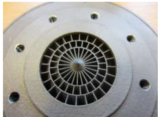
b: (part of the sodium channel) - realized by 3D prototyping technology
