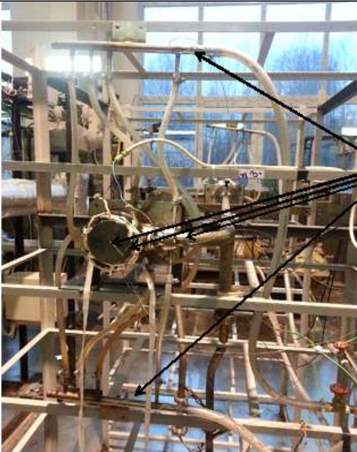
Figure 27 : The thermo acoustic loop with the locations of the thermocouples
