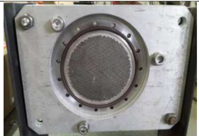
Figure 35: Graphite seals and O-rings All sealings in thermoacoustic generator has been made with high pressure stainless steel graphite sealings and with O-rings made from Viton material, made for high pressure.
