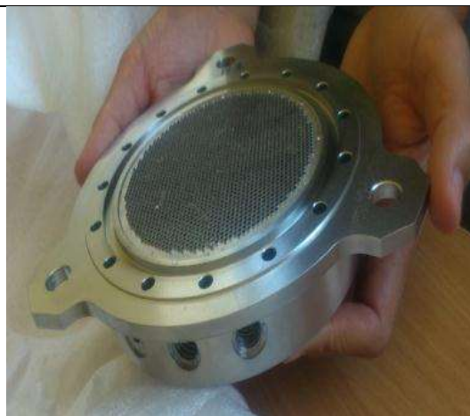
Figure 31: The cold exchanger
