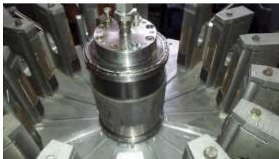
a: Module MHD partially mounted: core and titanium shell
