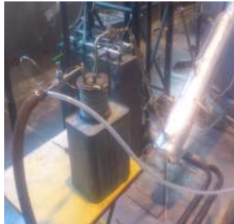
2) with heating system, vacuum pump and argon bottle connected
