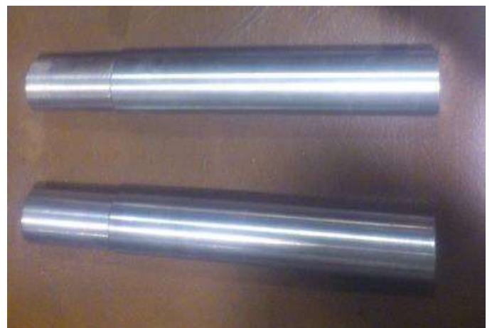
Figure 41: First elements of connection between the two actives parts of Thermo acoustic loop
