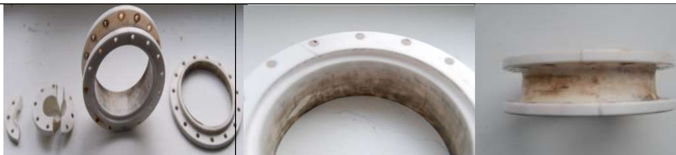
Figure 49: Rupture of the zirconium pieces
