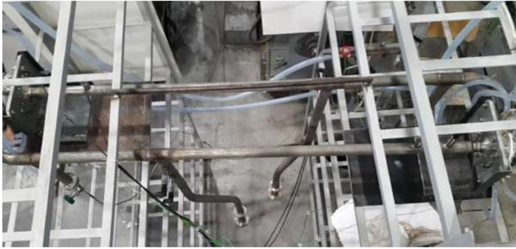
Figure 38 : Photo of the constructed thermos acoustic loop
