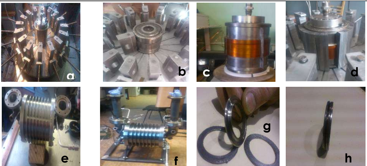
Figure 39: elements of construction of MHD generator
