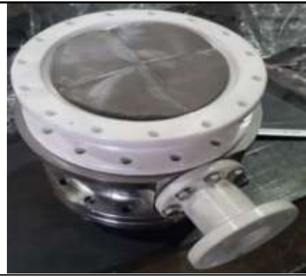
Figure 33: Zirconium flange Zirconium flange separates cold heat exchanger from hot heat exchanger. Inside zirconium flange there is a regenerator, which has been made by stack of steel. It consists of many steel plates, where heat can go from one plate to another.
