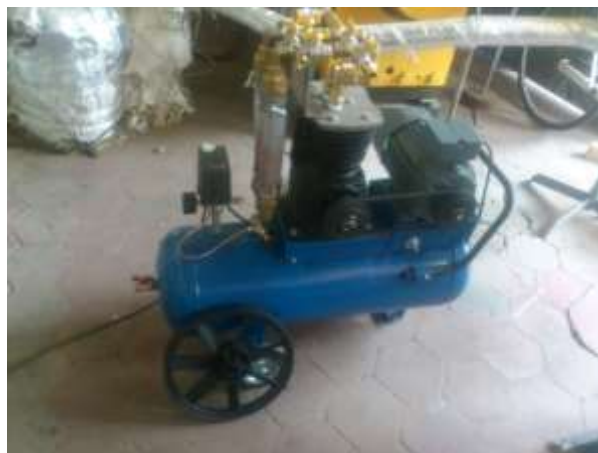
Figure 6: Compressor applied for pneumatic tests
