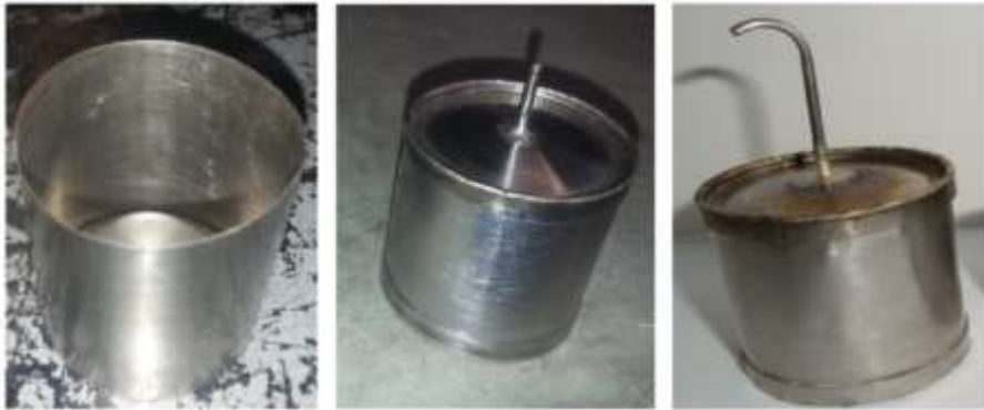
Figure 66: New type of floating piston with curved tube at the top.
