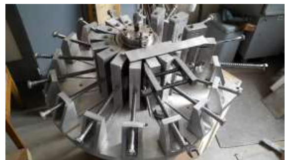
b: Module MHD partially mounted: yoke element positioned onto the magnets and the coils
