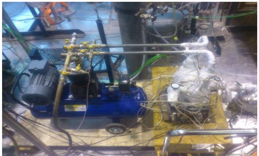
Figure 51: view of the test operation of the MHD generator actived by the compressor
