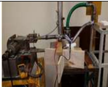
Graduation made in In-Ga-Sn eutectics loop using electromagnetic pump and Venturi tube
