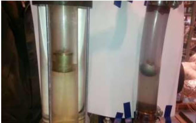
Figure 64 :View of the experimental device used to test the floating piston with water and Plexiglas tube
