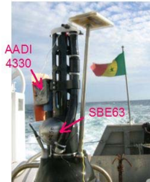
Figure 2.1.1: Navis float equipped with SBE63 sensor and 4330 optode.
