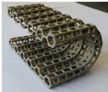
(b) Slurry impregnated template
