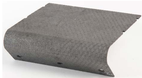
(c) C/C-SiC-HC leading edge for concept 1a
