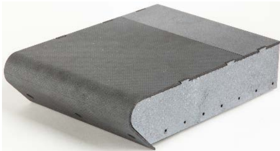
(b) C/C-SiC leading edge for concept 1b
