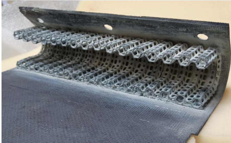
Figure 13: SiC/SiC leading with joined lattices.
