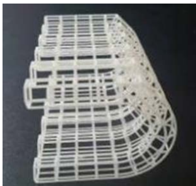
(a) 3D-printed polymeric template
