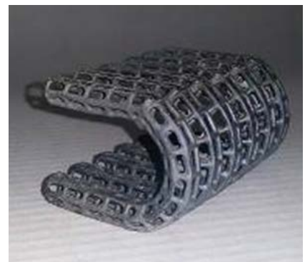
(c) Si-SiC lattice component after LSI
