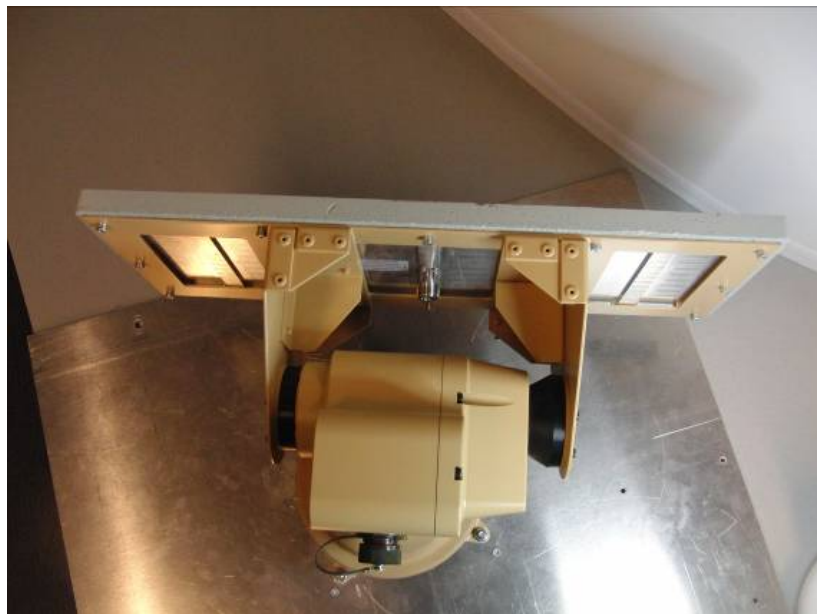
The MiniSAR PTU with flat panel microstrip RFA mounted on it
