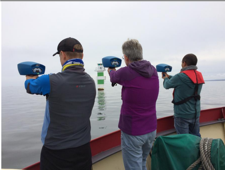
Figure 12, Radiometric comparison with three WISP-3's, the AERONET-OC station Palgrunden in the background
