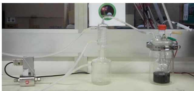
Figure 5.9 Sital's test bench for evaluating the catalytic activity of different materials/catalysts (left). Example of data acquired during a catalytic activity test (left): liquid temperature (black +), gas temperature (red x) and mass flow rate (green Δ).
