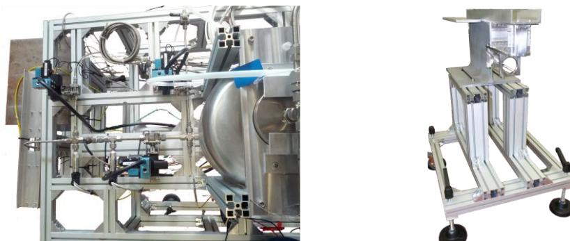
Figure 5.15 The fluidic line supporting structure (on the left) and the thrust balance (on the right) specifically designed for assessing the propulsive performance of the PulCheR monopropellant propulsion system.
