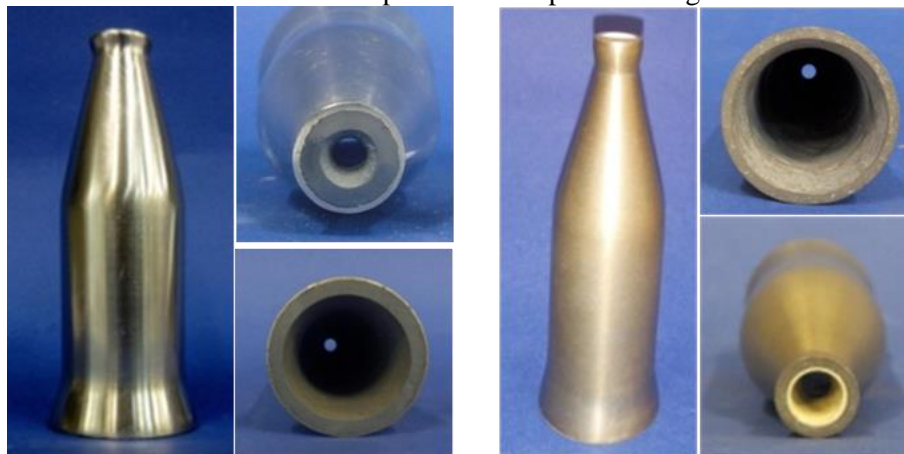
Figure 5.23 The two types of combustion chambers developed and manufactured by Demokritos. On the left the SiC-based combustion chamber with the outer layer made of Molybdenum. On the right the ZrO 2 -based multilayer material.
