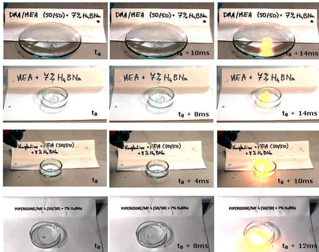
Figure 5.26 Drop tests of the fuels promoted by hydride additives on HTP.
