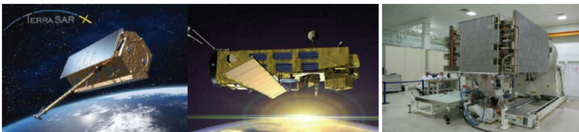
Figure 1. Representative SAR instruments (by ESA). Terrasar-X (left), ENVISAT (center) and COSMO-SkyMed (right)
