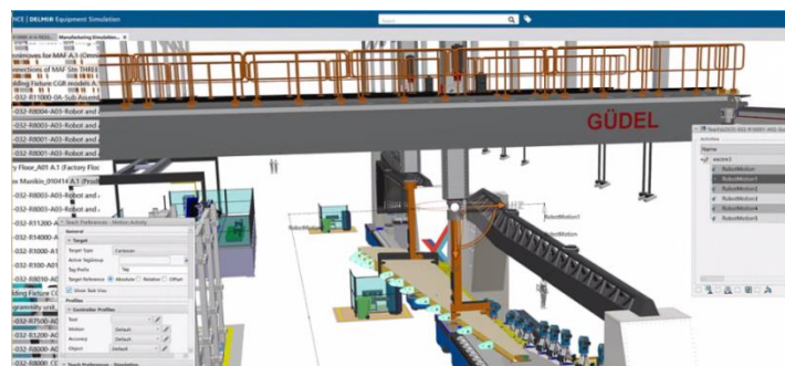
Figure 46. The Handling of the wing is simulated through the production line
