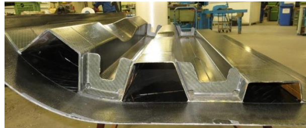
Figure 20. Composite panel with cocured skin, stiffeners and shear clips
