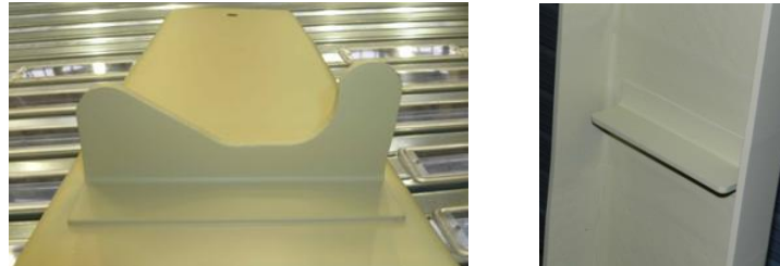
Figure 21. Locomachs Rear Spar with cocured hinge attachment
