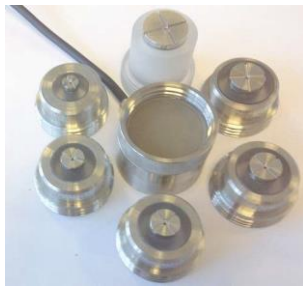
Figure 29. Set of Daisy matrix probes by AGI for countersink inspection Figure 30. DASSAV's linear Array
