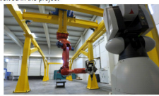
MEGAROB main elements: Laser tracker, robot and structure
