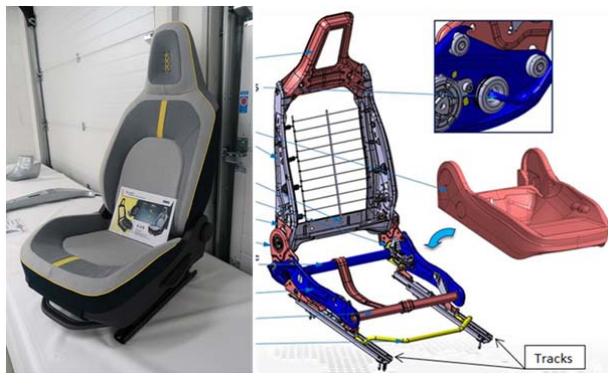
Fig. 7 Light weight seating concept (Faurecia)
