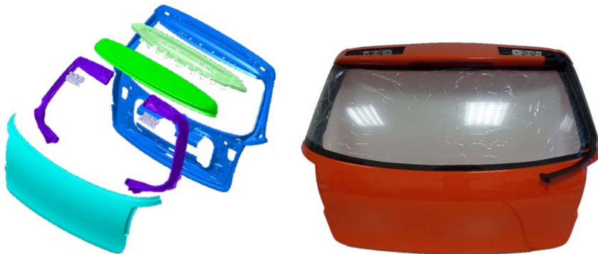
Fig 29 Exploded view of the prototype tailgate (left) and the final assembly (right).
