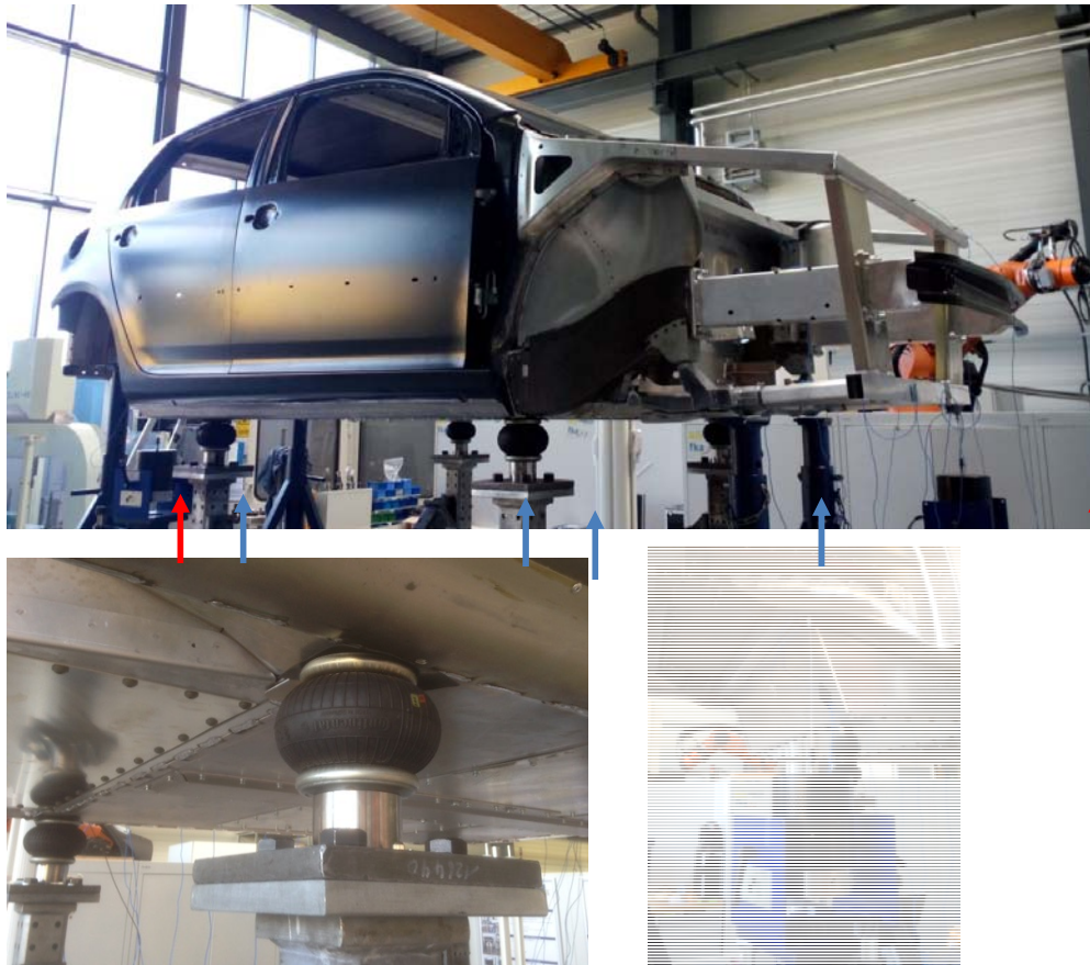
Figure 24: BiW with doors on the test rig. Suspended by 4 air springs (blue arrows, zoom bottom left) and 2 excited by 2 shakers (red arrows, zoom bottom right)
