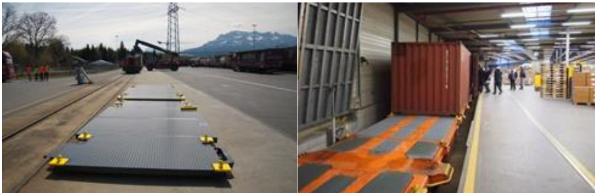
Container Loading Adapter (left picture) and Flex Freight Car with iron grid inlay (right).
