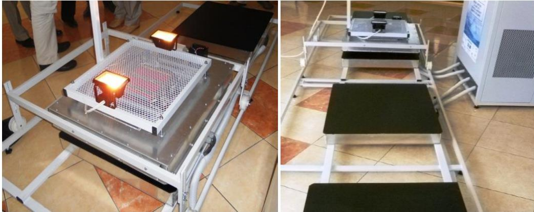
Figure 2 - Mock up for static and on-route inductive charging performance test and analysis
