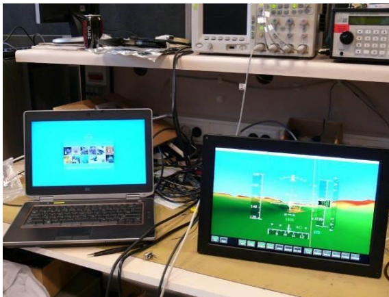
Figure 2.4.2.2 DHA on the test bench
