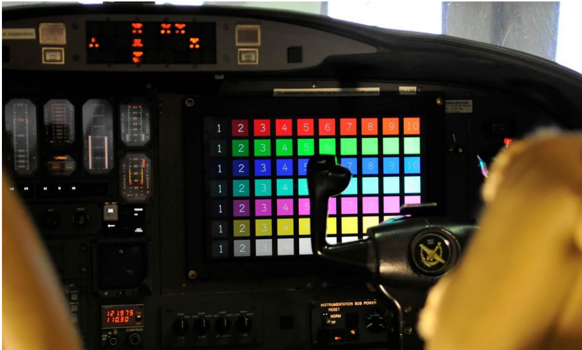
Figure 2.6.1.2. DERPHOSA display with test pattern
