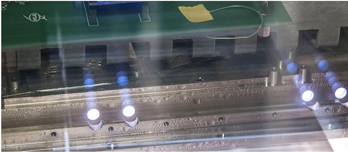
Figure 2.5.5.4 Post Condensation test
