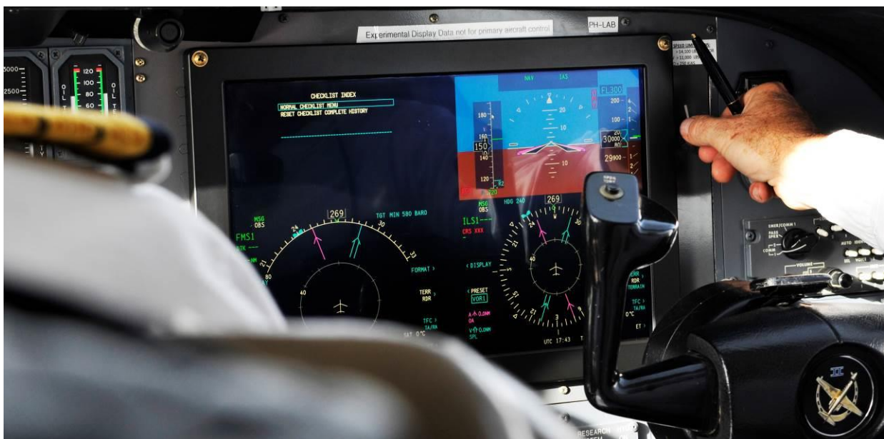
Figure 2.6.1.1. DERPHOSA display in NLR's Citation II cockpit
