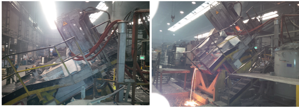
Figure n° 19.- General view of plasma torch device mounted on the big tundish
