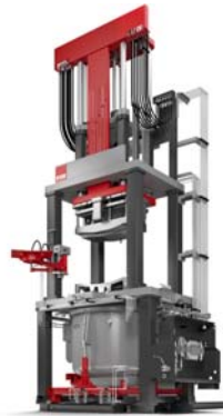
Figure 28: LPSC demonstrator based on a LOW PRESSURE CASTER W by FILL
