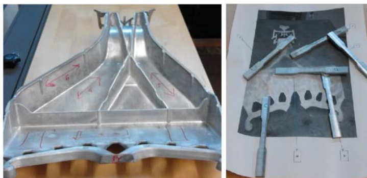
Figure 14: Tensile test bar extraction from SCMg part.
