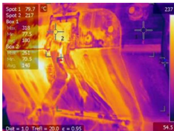
Figure 5: Thermal control of die's temperature with a thermocamera.
