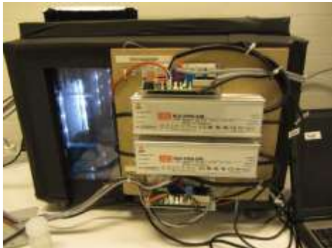
Figure 11: Ice test chamber (sample plate is visible to the left).
