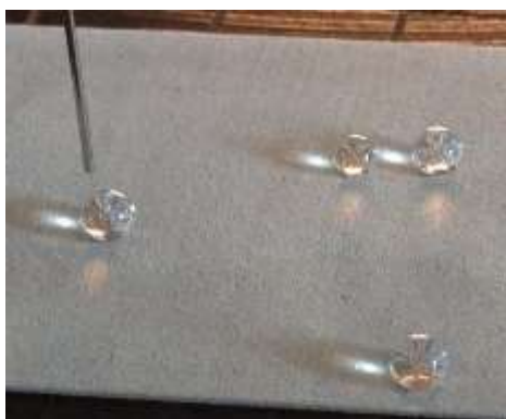
Figure 8: Water drops rolling off a dry superhydrophobic surface.
