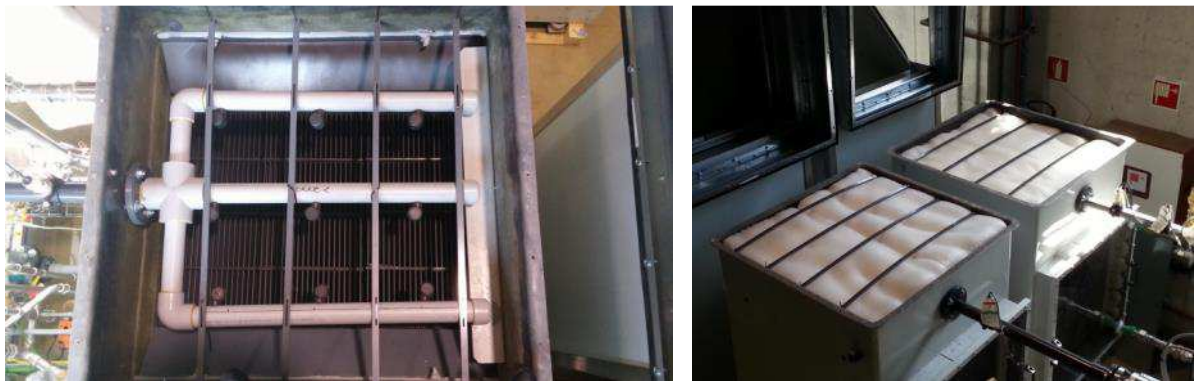
Figure 12. Distributor with nozzles (left) and demisters of the absorber and regenerator towers (right)
