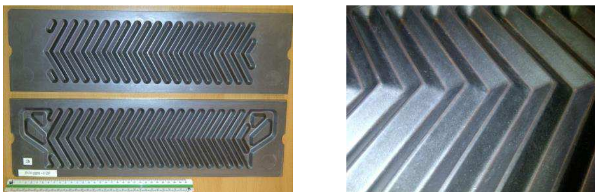
Figure 9. PHE plate made of 22% PP, 74% Graphite and 4% GNP
