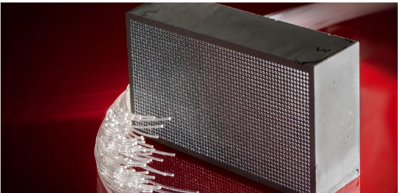
Figure 4.1.8. Concrete and light guide screen.
