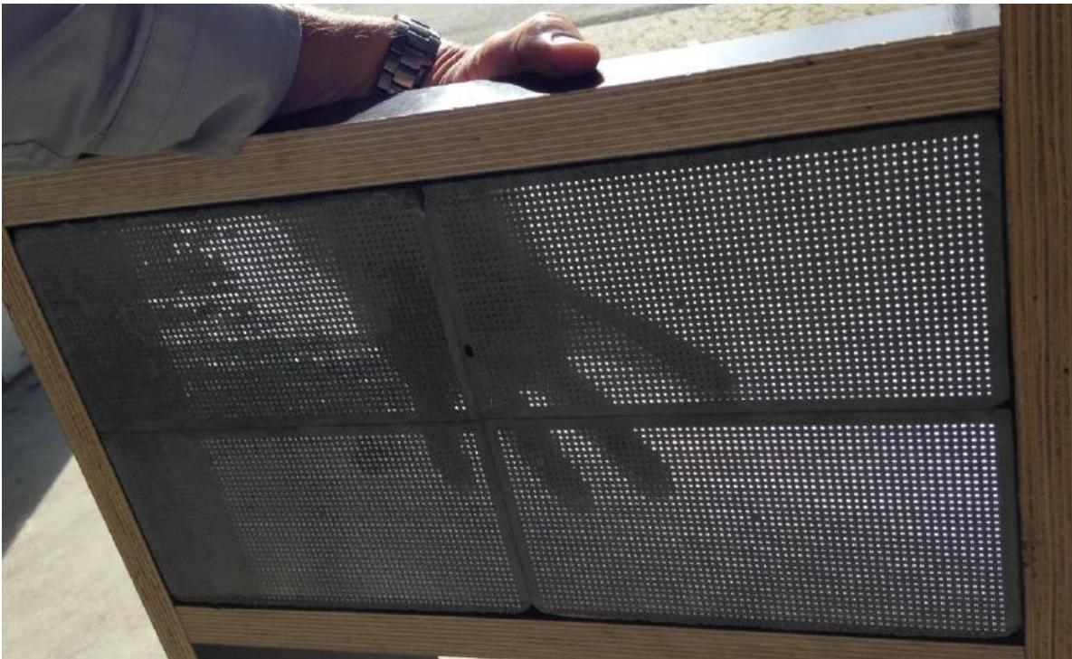
Figure 4.1.9. The four transparent concrete and light guide screens were arranged in a frame in order to make the final screen of the prototype.
