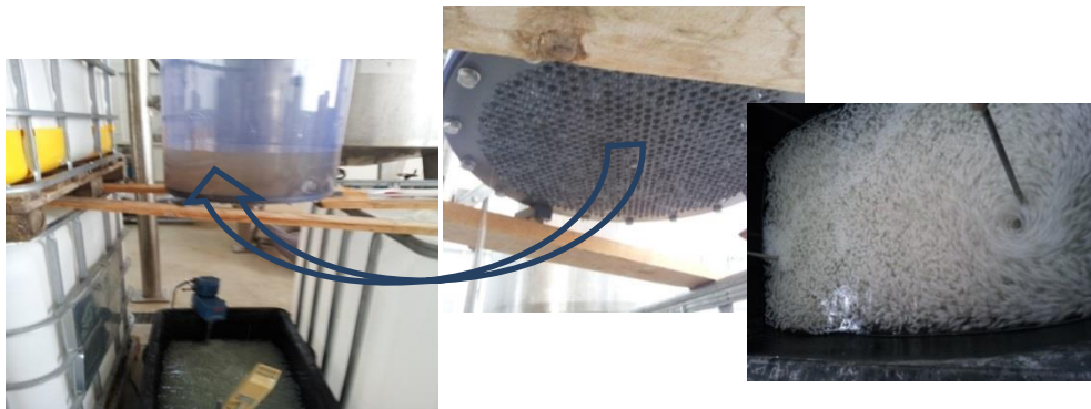
Fig. 4. Beads formation in NaOH solution
