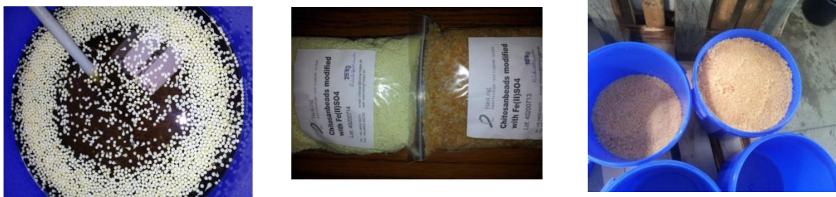
Fig. 7. Beads modification with iron sulphate solution
