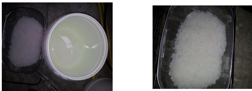
Fig. 5. Washing of chitosan-beads
