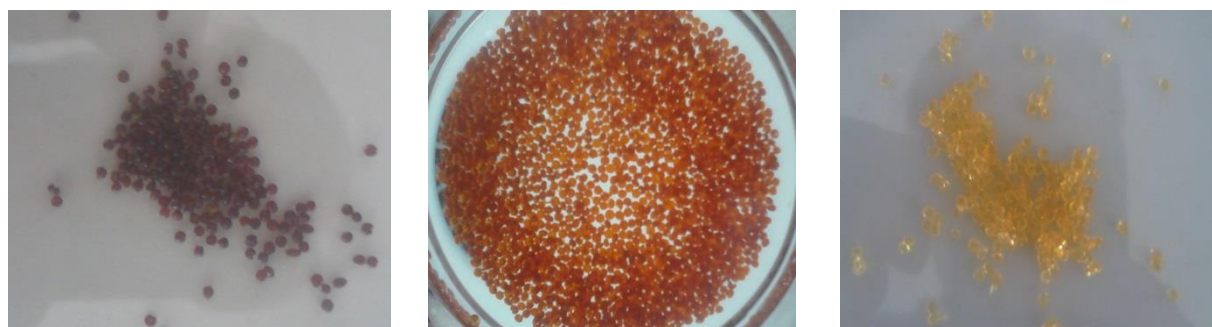
Fig.20 . FTMC beads: a) unloaded; b) loaded with metals and pesticides; c) regenerated
