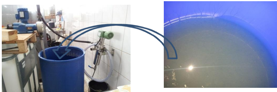
Fig. 3. Dissolution of Chitosan into citric acid solution
