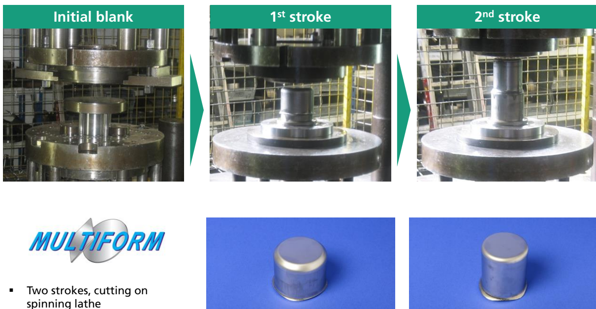
Figure 9: Manufacture of reference components by deep drawing
