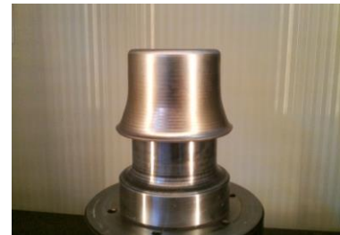
Figure 10: Manufacture of reference component by conventional spinning with intermediate annealing
