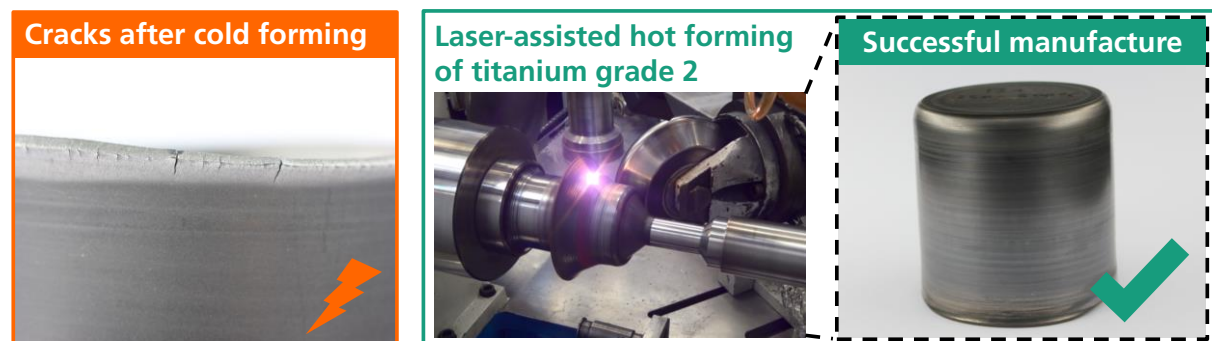
Figure 6: Laser-assisted metal spinning facilitates crack-free manufacture of titanium demonstrator
