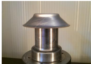
Figure 10: Manufacture of reference component by conventional spinning with intermediate annealing
