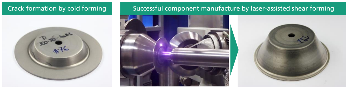
Figure 3: Laser-assisted shear forming of titanium grade 2 facilitates successful component manufacture in contrast with cold shear forming
