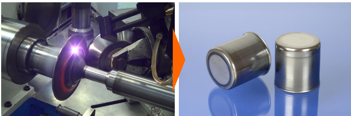
Figure 11: EasyForm demonstrators manufactured by laser-assisted spinning
