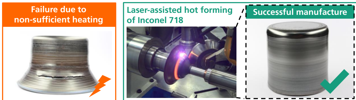
Figure 5: Laser-assisted metal spinning facilitates successful manufacture of Inconel demonstrator in contrast with cold forming
